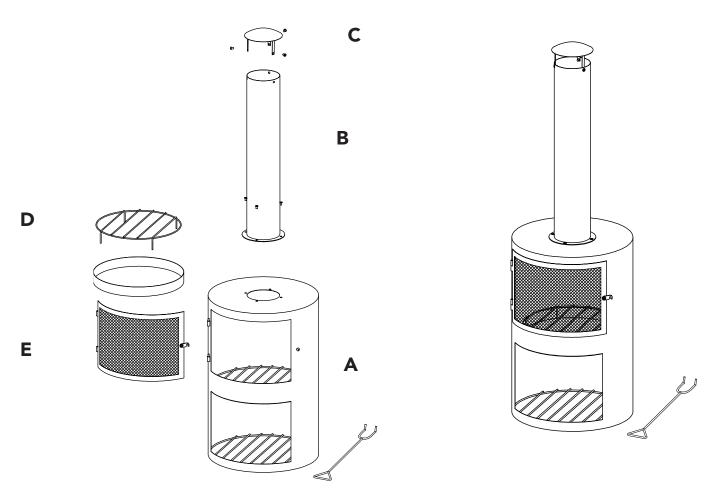
Stap 1: Connect the Base (A), the chimenea (B) and the raincap with the bolts and nuts.Stap 2: Put the woodgrid (D) and the sparkscreen (E) into the base (A).
